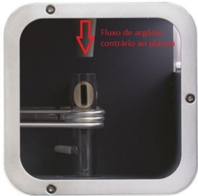
Figure 4. iCAP PRO Series ICP-OES duo torch box with inner torch box mounted
